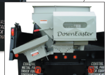
Optional flip chute detaches by taking out 2 pins. Tow a trailer while the sander is on your truck. Great for emptying the hopper, and off-season storage.
